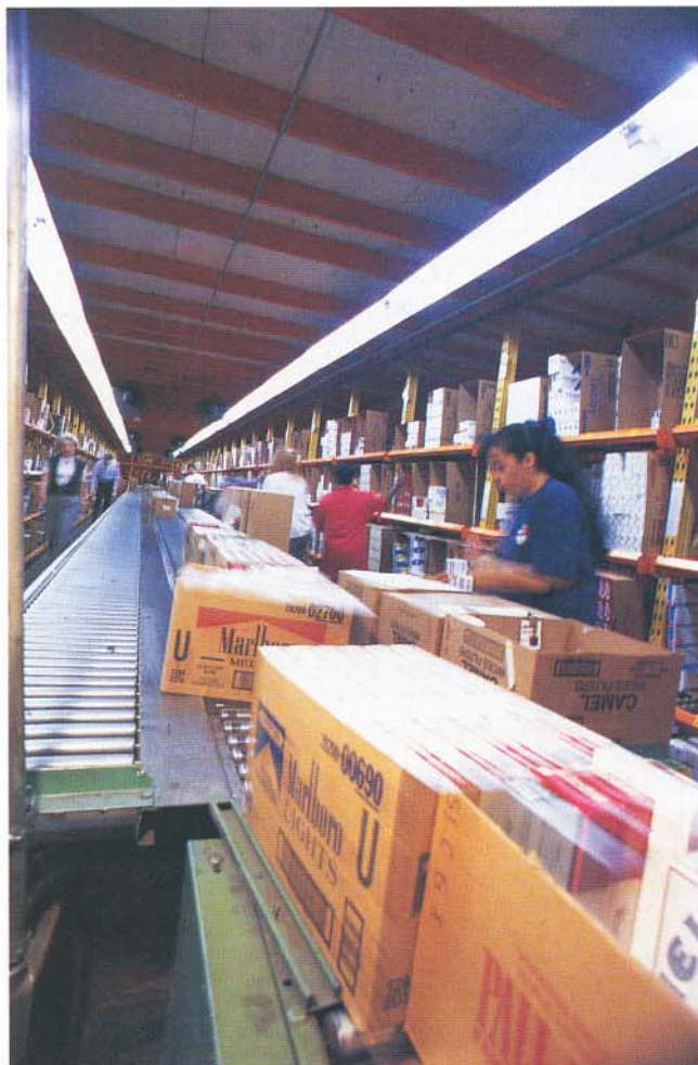
THE RIGHT PRODUCT AT THE RIGHT TIME: A common use of AS/RS is in the support of manual picking operations.
