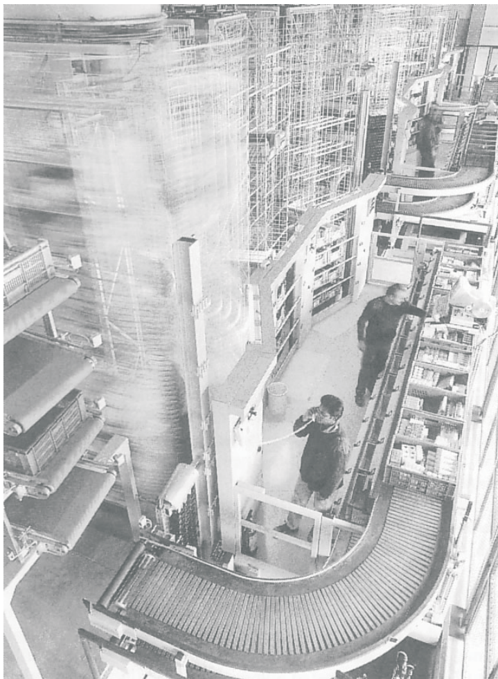
An overhead view at Albert Heijn gives a good indication of the carousel workstation arrangement at the Geldermalsen facility. Orders are batch processed twelve at a time. Selection rate is in the approximate 430-450 pieces-per-hour range.
